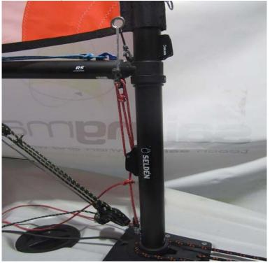
This downhaul system requires 1 extra block (so 2 in total), 2.5m of 4mm line, and a further 60cm of 4mm line at the top. If the easy rig option is required it is 40cm of 3mm line and a rope bobble or big knot in the end. (a rope bobble is considered a knot in a rules interpretation). This is knotted through the gooseneck moulding and round the mast for strength.
