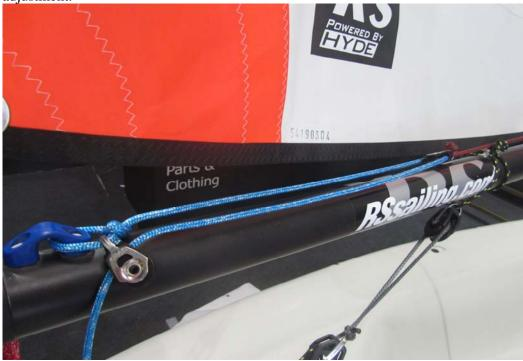
This requires 3 of 20mm block and 2 lengths of 4mm line of 2meters each. A further lashing for the rear block is required. This is available as a kit for £22.
